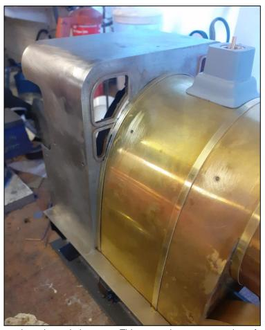
Then onto the cab, again laser cut. This comes in two parts, cab roof, sides and the cab front. The cab roof requires two bends in it to make the sides. The two pieces are then riveted together using 1/4" brass angle. I finally ran a bit of solder around the edge to fill any slight gaps.
