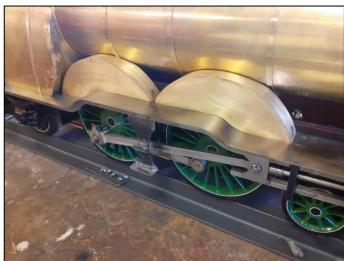
boards required bending to shape to match the profile of the stiffener strip that goes on the underside.
