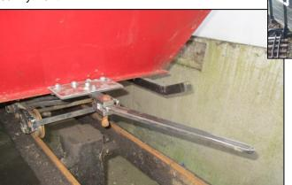
Dave has completed a new coupling and fitted them to the red ball wagon. They've been tested and worked perfectly.
